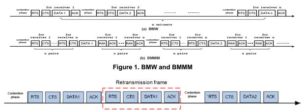
Figure 2. Retransmission frame structure in BMW
